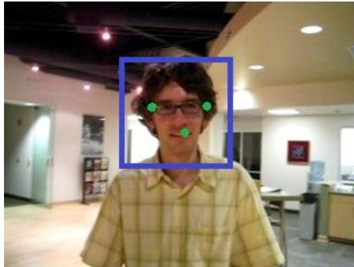
Figure 4.2: Frame of image sequence where pyramidal lucas-kanade is applied to follow the green points inside the bounding box. This image is part of VOT2014 Dataset [37]
