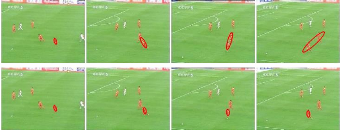
Figure 2.3: Player tracking, first row- CAMSAHIFT tracker, Second row- Kalman Filter with CAMSHIFT algorithm [8].
