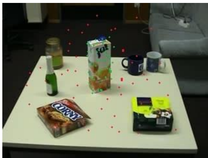
Figure 5.4: Image keypoints. Green dots represents the foreground keypoints, red dots represents the background keypoints.
